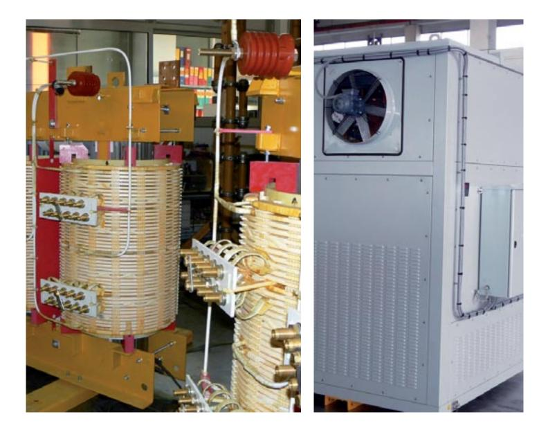
Distribution transformers MV/MV, MV/LV and LV/LV type for energy distributions in our production range are dry type AIR FILLED, with AN or AF (or combined) cooling method, class H or F, in accordance with E0, F0 and C0 class.
