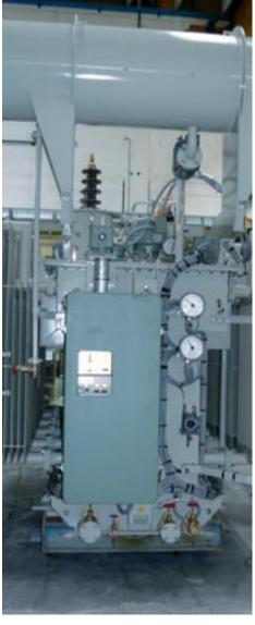
Distribution transformers MV/LV type for energy distributions are usually three or single phase, oil immersed, with different cooling method (K/L)ONAN - (K/L)ONAF with detachable radiators or corrugated tank (depending on transformer size and ambient temperature), with conservator technology or sealed construction (with or without nitrogen / air filling).
